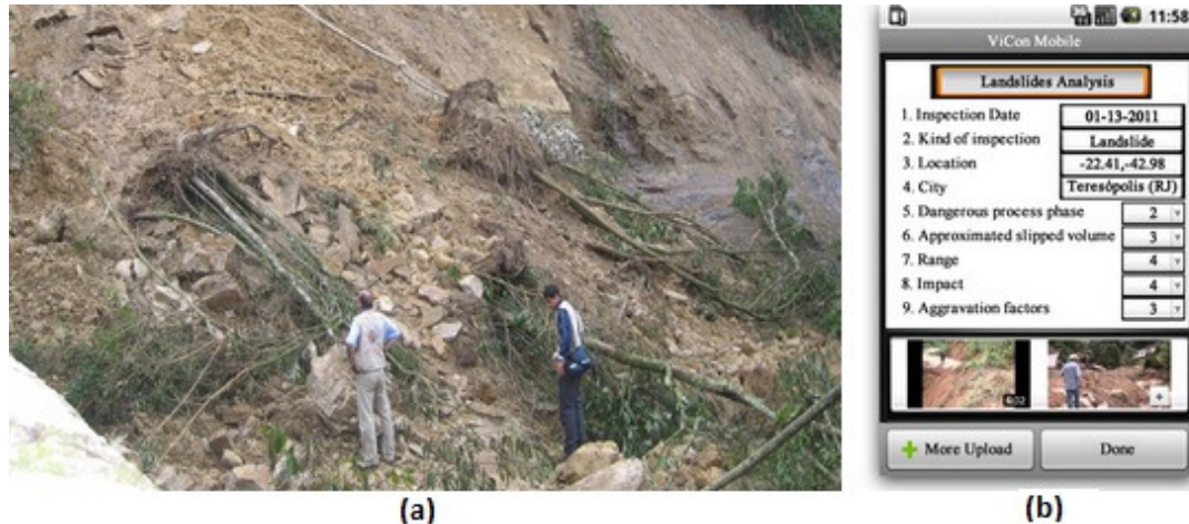
Figure 2. Landslides assessment by CENACID members in Teresópolis - Brazil (2011) and Data Gathering Platform (under development) (b)
